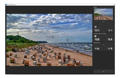
The sensor spot corrector marks all of the patches and determines a source within the image that can be used as a substitute.
