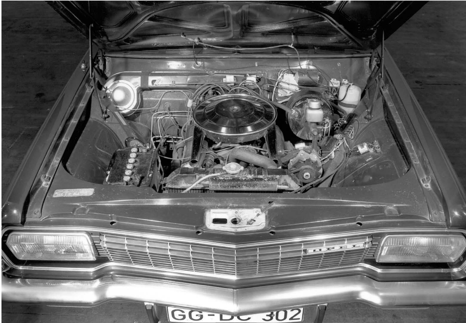
Der Opel Diplomat besaß einen V8-Motor aus dem Baukasten der Konzernmutter General Motors. The Opel Diplomat had a V8 engine from the construction kit of the parent company General Motors.
